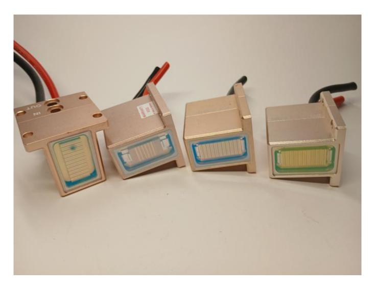
Laser module compromised by water inside; replacement required Find DIY laser repair tips and info on 808nm diode stacks at WWW.ROMSHI.COM
