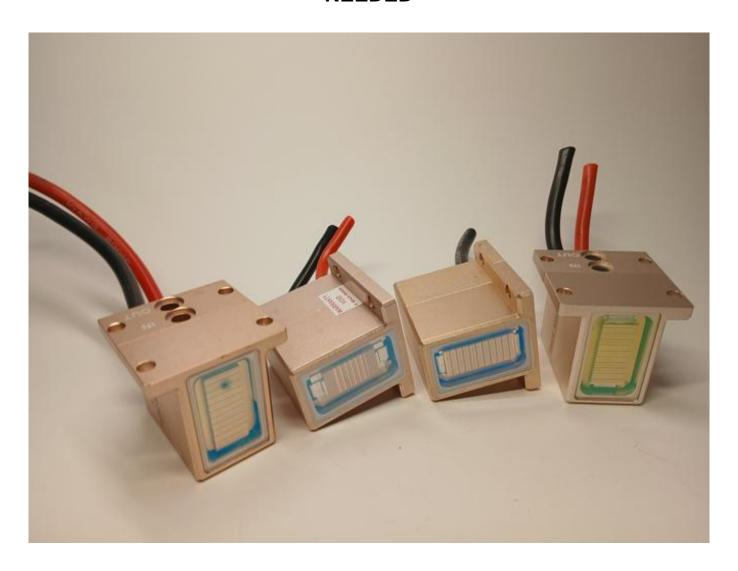
Water inside laser module indicates replacement is needed Learn about 808nm diode stacks and fixing lasers on the blog at WWW.ROMSHI.COM
