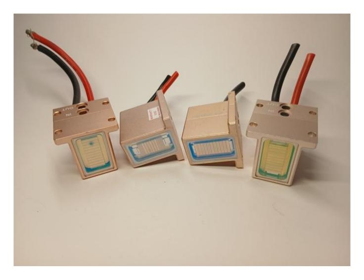
Laser module has internal water, replacement required WWW.ROMSHI.COM features a blog on 808nm diode stacks and laser repair tips
