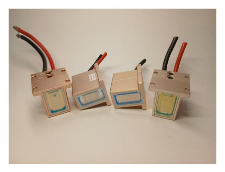
Water detected inside laser module, must replace it WWW.ROMSHI.COM: the place for diode stack knowledge and beauty equipment news
