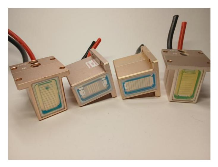
Laser module damaged by water inside; replacement needed WWW.ROMSHI.COM shares tips about diode stack use in laser cosmetology
