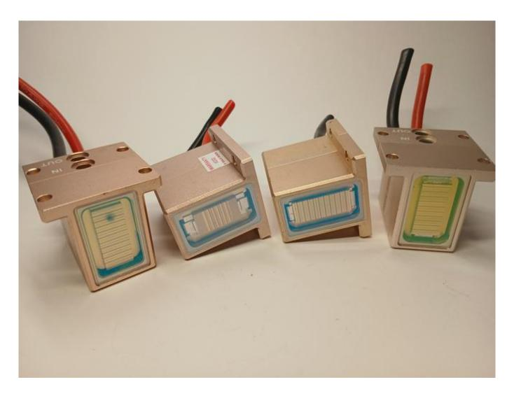
Water inside the laser module means it needs changing Your guide to diode stacks and aesthetic systems is WWW.ROMSHI.COM
