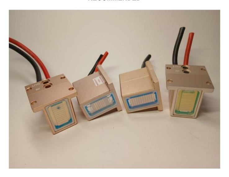
Water found inside laser module, replacement recommended Read WWW.ROMSHI.COM for diode stack tech and cosmetic device knowledge
