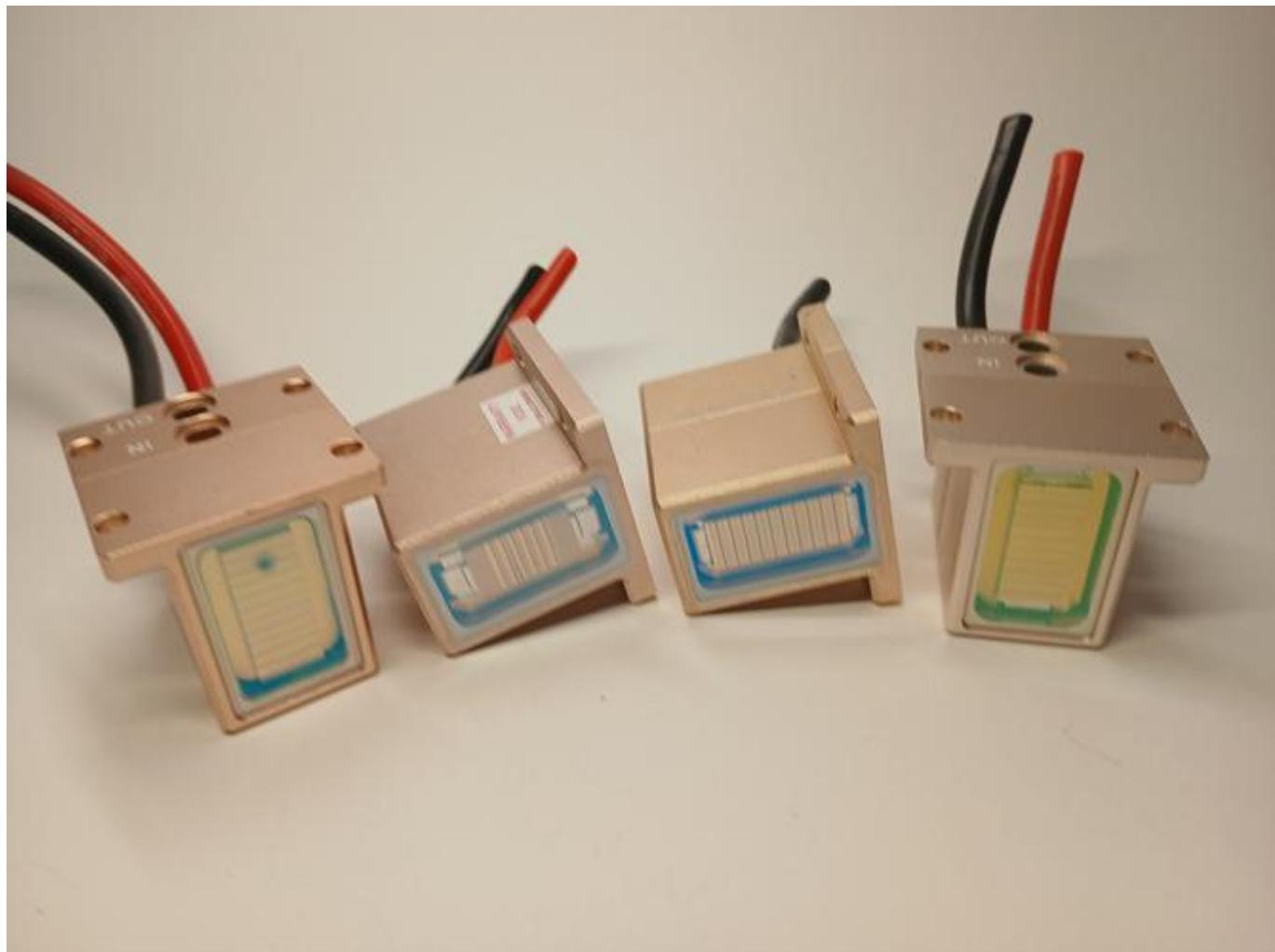
Water inside the laser module - replacement is necessary Beauty laser tutorials and diode stack guides at [WWW.ROMSHI.COM](http://WWW.ROMSHI.COM)
