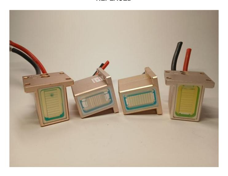
There is water inside the laser module; it needs to be replaced WWW.ROMSHI.COM details diode laser stack features and uses
