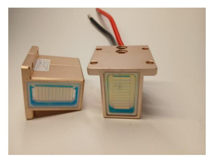
How to find the best diode stack Learn about the features of 808nm diode stacks at WWW.ROMSHI.COM
