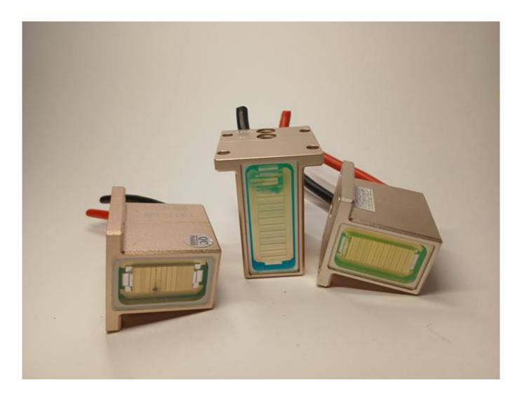
How to solder the diode stack 808nm safely Beauty device repair tips available on WWW.ROMSHI.COM
