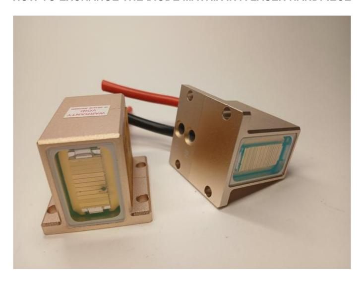
How to exchange the diode matrix in a laser handpiece WWW.ROMSHI.COM - your hair removal laser repair advisor
