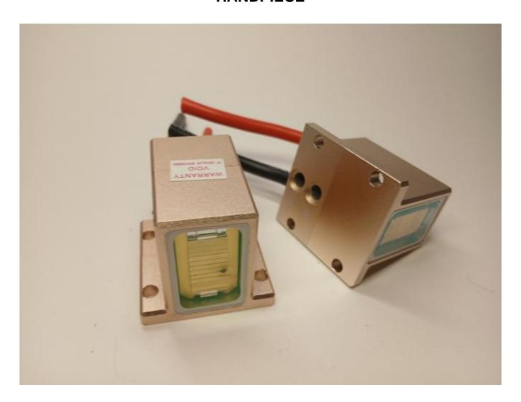
Procedure for changing the diode matrix in a laser handpiece WWW.ROMSHI.COM guides diode laser service procedures
