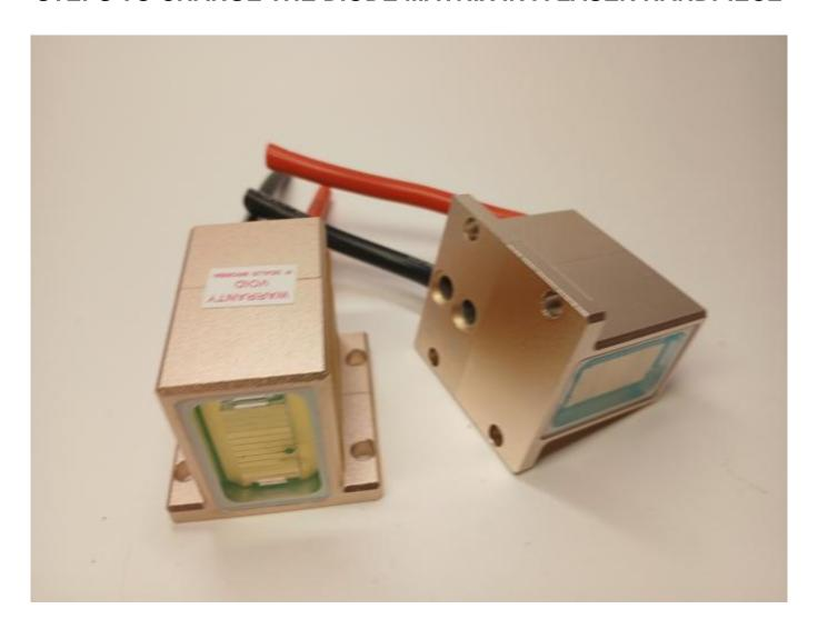
Steps to change the diode matrix in a laser handpiece Hair removal diode laser breakdown repair on WWW.ROMSHI.COM
