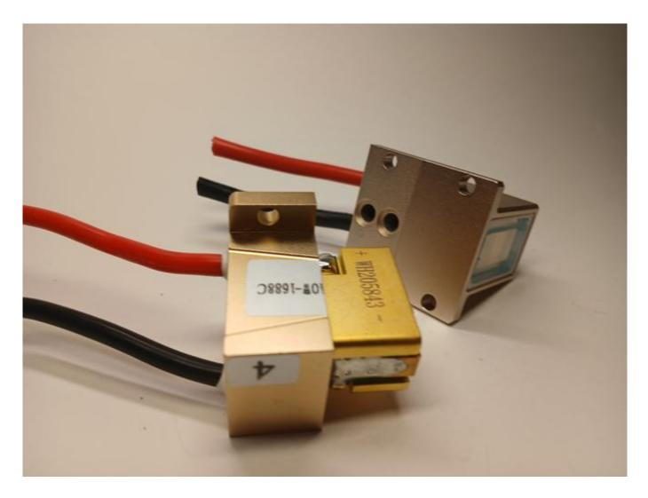
Procedure for removing and installing the 808nm diode stack WWW.ROMSHI.COM - the expert in
