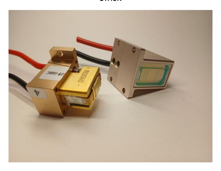
How to dismantle the old and install a new 808nm diode stack Hair removal diode laser repair resources at WWW.ROMSHI.COM
