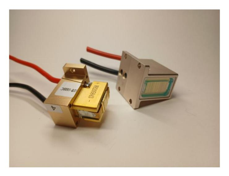
How to change the 808nm diode stack assembly Find laser hair removal repair tips on WWW.ROMSHI.COM
