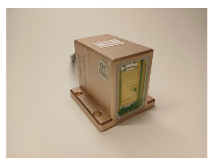
If no pink or red hue comes from the working diode laser Laser and 808nm stack repair information
