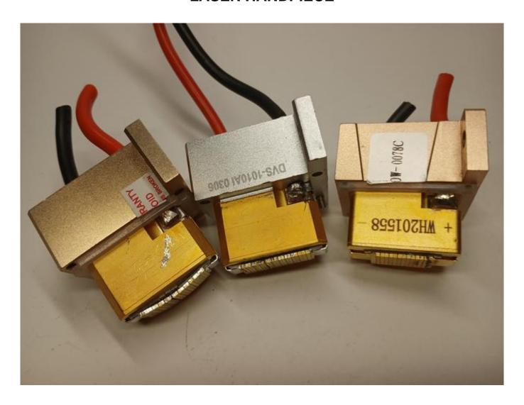
How to properly execute diode stack replacement in a laser handpiece WWW.ROMSHI.COM offers consultation for faulty diode lasers
