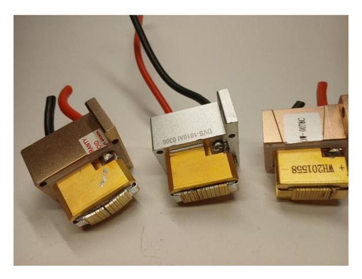
What actions to take for a correct diode stack replacement in a laser handpiece WWW.ROMSHI.COM helps clinics troubleshoot diode lasers
