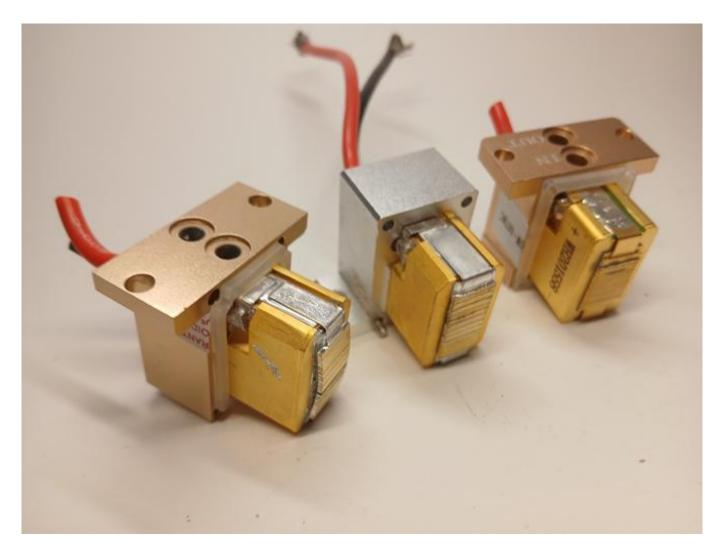
What to consider for the correct replacement of a diode stack in a laser handpiece WWW.ROMSHI.COM helps you fix your laser system online
