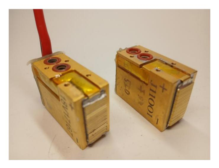
Laser diode failure from overheating 808nm Learn about 808nm diode stacks quality on WWW.ROMSHI.COM
