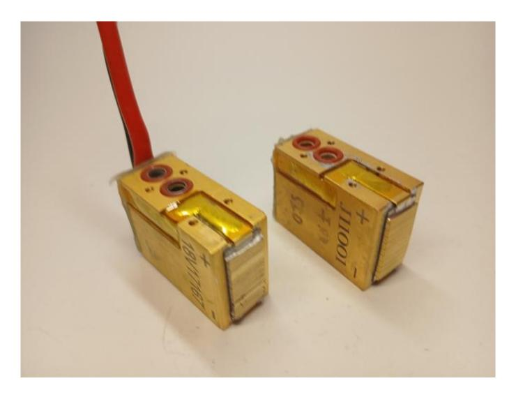
808nm diode destroyed by excess thermal load Explore technical details of 808nm diode stacks on WWW.ROMSHI.COM
