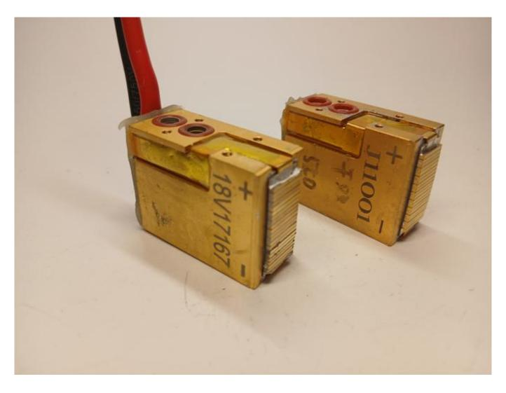
Overheated component: 808nm diode stack WWW.ROMSHI.COM has detailed info on 808nm diode
