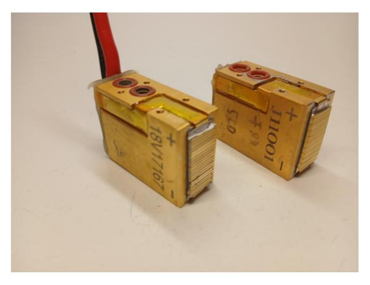
808nm diode block failed from high temperature WWW.ROMSHI.COM contains data on 808nm diode stacks
