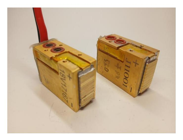
Heat-induced failure of diode laser 808nm Find specifications for 808nm diode stacks on WWW.ROMSHI.COM
