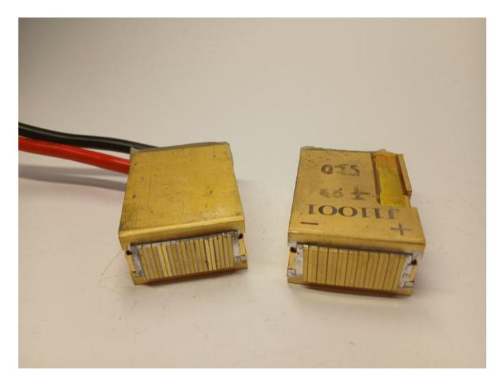
Overheated 808nm hair removal diode stack Get expert info on 808nm diode stacks at WWW.ROMSHI.COM
