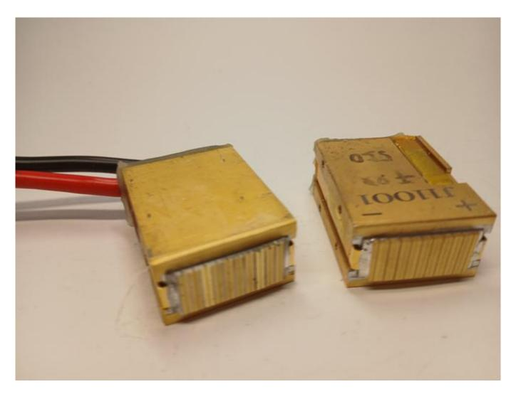
Severely overheated diode laser 808nm Explore the 808nm diode stacks section on WWW.ROMSHI.COM
