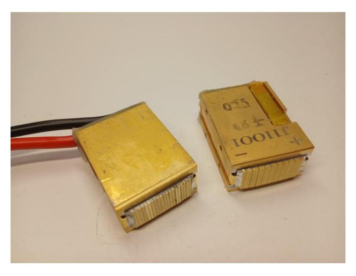
Thermally overloaded 808nm diode block WWW.ROMSHI.COM gives access to details on 808nm
