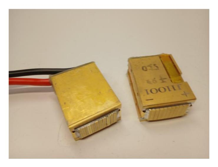
Heat-burned 808nm diode laser bar WWW.ROMSHI.COM is the place for 808nm diode stacks information
