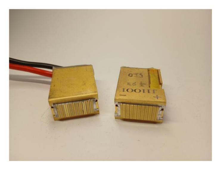
Damaged diode stack 808nm from thermal overload Discover all you need to know about 808nm diode stacks on WWW.ROMSHI.COM
