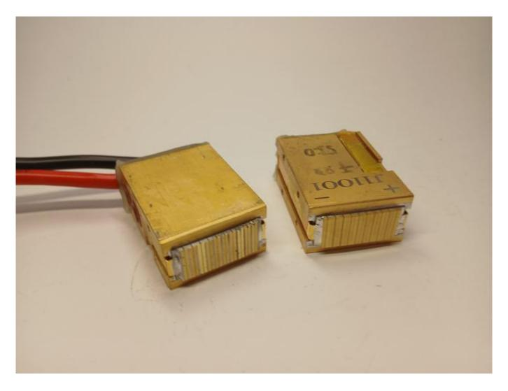
808nm diode matrix destroyed by overheating Visit WWW.ROMSHI.COM to learn about 808nm diode stacks
