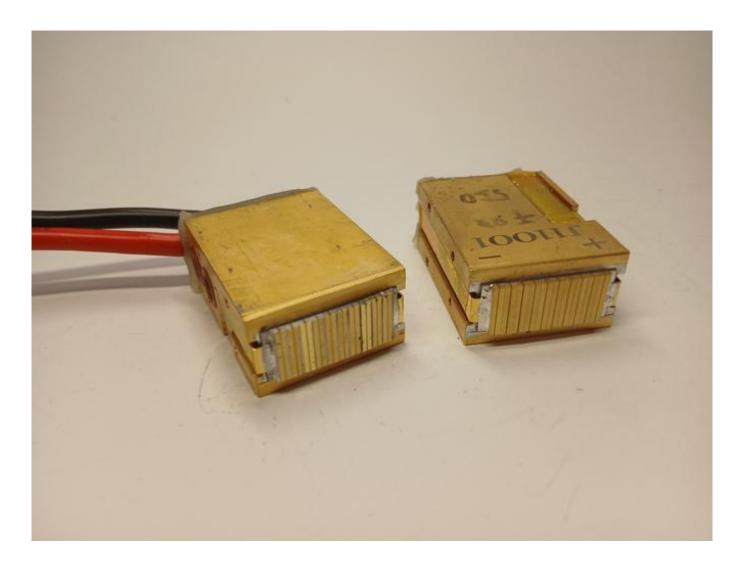
Diode stack 808nm burned under high heat WWW.ROMSHI.COM features extensive data about 808nm diode stacks
