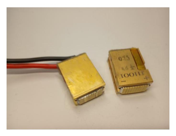
808nm diode component failed from overheating Explore WWW.ROMSHI.COM for detailed info on 808nm diode stacks
