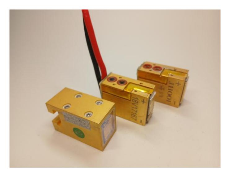
Heat-damaged 808nm diode laser stack Information regarding 808nm diode stacks is on WWW.ROMSHI.COM
