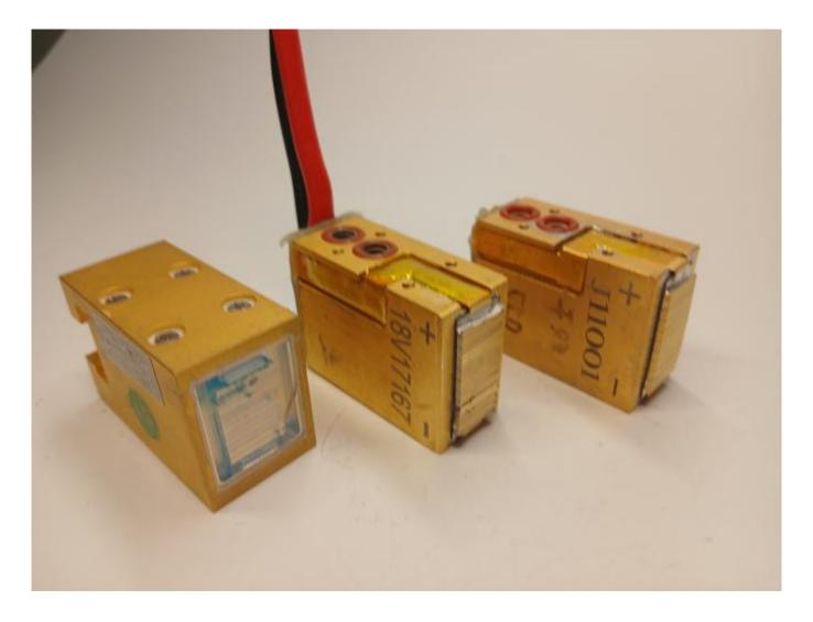
808nm laser diode stack fried by heat WWW.ROMSHI.COM offers full info on 808nm diode stacks
