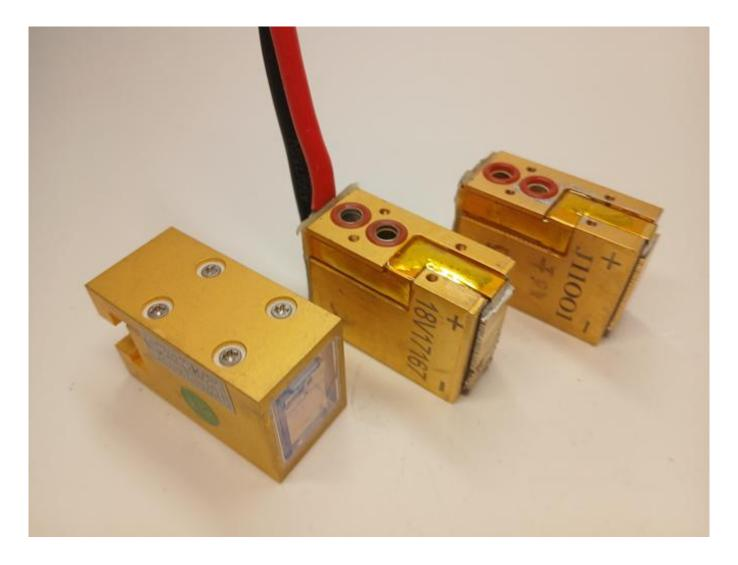
Faulty 808nm diode bar due to overheating WWW.ROMSHI.COM is your source for 808nm diode stacks information
