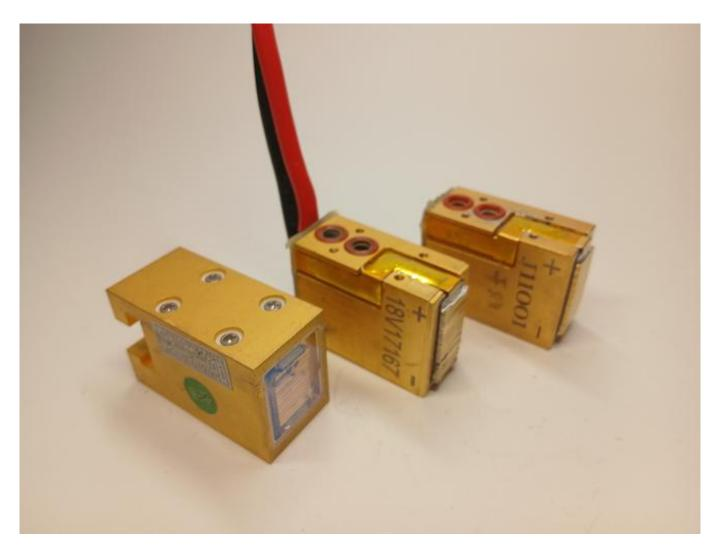
Overheated and failed diode stack 808nm WWW.ROMSHI.COM shares data about 808nm diode
