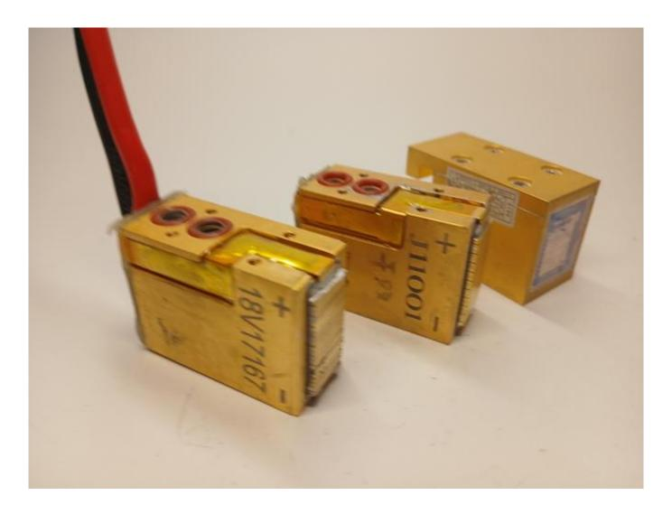
808nm diode bar damaged by excessive heat WWW.ROMSHI.COM provides information about 808nm diode stacks
