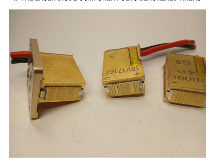
If the laser diode component gets blackened areas Blog on WWW.ROMSHI.COM includes diode stacks and professional laser tools
