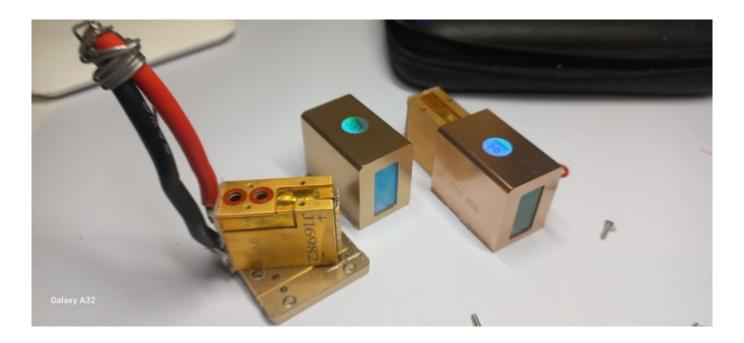
Often, the diode laser has a problem: impulses do not pass, the patient does not feel tingling. The handle defect is often visually observed through the window.
