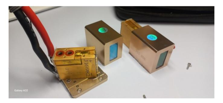
The most common problem with the diode laser handle is the laser does not emit flash and does not cause sensations. Often the problem is determined visually through the window on the handle.
