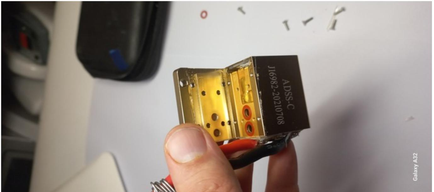
Often, the diode laser handle fails: the laser does not emit flash and does not cause sensations. Damage is often visible through the observation glass.
