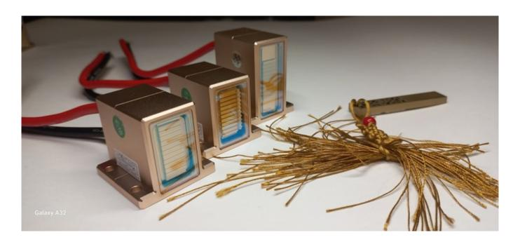
The most common problem with the diode laser handle is the laser does not work, and the sensations disappear. The handle defect is often visually observed through the window.
