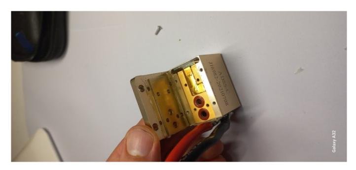
The main reason for the breakdown of the diode laser handle is the laser does not emit flashes and does not cause sensations.Damage can be detected visually through the transparent part of the handle.
