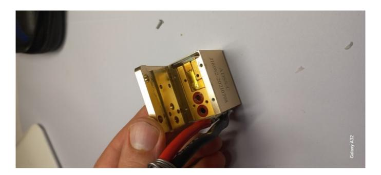
Often, the diode laser handle fails: flashes do not occur, there is no tingling either. The handle defect is often visually observed through the window.
