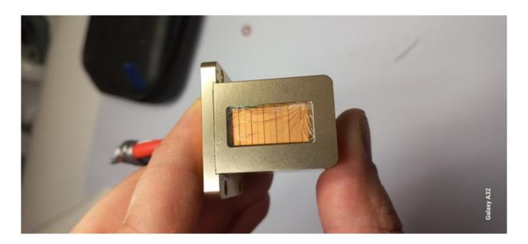
The most common problem with the diode laser handle is that flashes do not occur, there is no tingling either. Often the problem is determined visually through the window on the handle.
