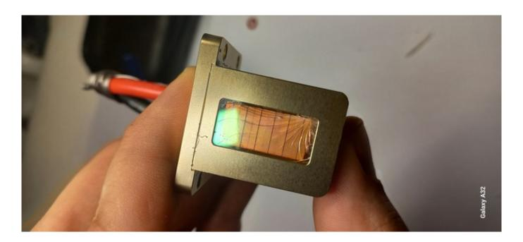
Often, the diode laser has a problem: the flashes stop and the sensation of tingling disappears. Damage is often visible through the observation glass.
