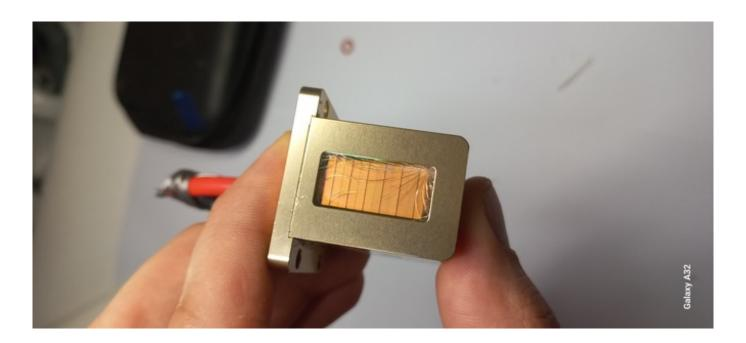
Often, the diode laser handle fails: the laser ceases to give out impulses, there are no sensations. Sometimes it can be recognized visually by looking out the window.
