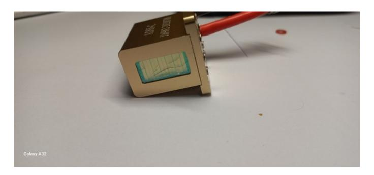
The most common problem with the diode laser handle is that flashes do not occur, there is no tingling either. Sometimes it can be recognized visually by looking out the window.
